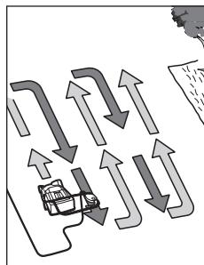
Place the product on the edge of the lawn, as close to the mains socket as possible. Work away from the mains socket.
